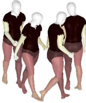
Figure 1. SCAPE from images. Detailed 3D shape and pose of a human body is directly estimated from multi-camera image data. Several recovered poses from an image sequence of a walking subject are shown.
