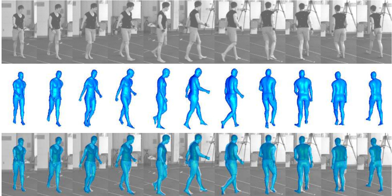
Figure 6. First row: Input images. Second row: Estimated mesh models. Third row: Meshes overlaid over input images. By applying the shape parameters recovered from 33 frames to the template mesh placed in a canonical pose, we obtained a shape deviation per vertex of 8.8 \pm 5.3mm , computed as the mean deviation from the average location of each surface vertex.
