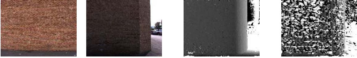
Figure 10: Left: two video frames, middle: gain corrected stereo, right: standard stereo.
