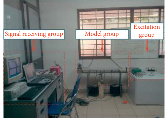
FIGURE 3: Experimental model of travel load on beams (obtained from LAM).
