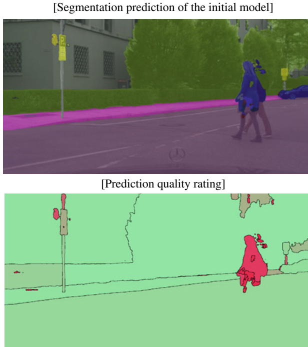
Fig. 4 Predicted semantic segmentation mask of the initial model’s prediction (top) and corresponding segment-wise quality estimation (bottom) for one example from the Cityscapes test split. Green color indicates a high segment-wise IoU, red color indicates a low one
