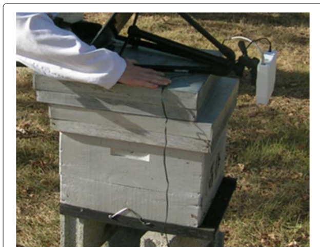
Figure 2 Stereo vision camera. A stereo vision camera capturing the entry of a beehive including the entire flight board.
