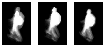
Fig. 5. Edge correlation temporal template over 15 \times 15 (left) and 30 \times 30 (middle) search windows. ICP temporal template (right) does not require any parameters.
