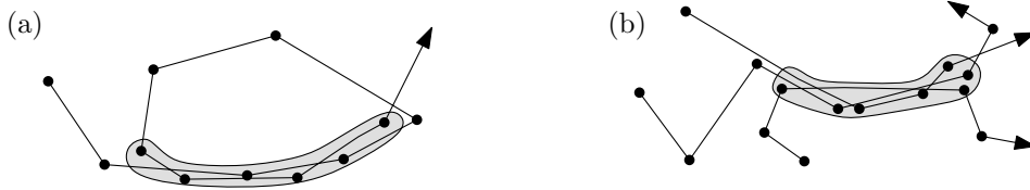
Figure 1: (a) The two subtrajectories within the shaded region form a subtrajectory cluster for m = 2 if the length of the longest subtrajectory is longer than \ell and the Fréchet distance between the two subtrajectories is at most d . (b) Illustrating a subtrajectory cluster for m = 3 in the case when a set of trajectories is given as input.
