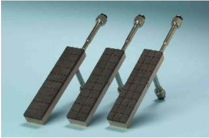
Figure 1: Pre series II divertor target elements.
