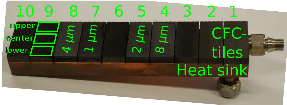
Figure 8: Example of a prototype of the W7-X divertor target element. It consists of 10 CFC tiles (with a thickness of 8 mm, a length of \approx 25 mm and a width of \approx 55 mm) bonded to a water-cooled CuCrZr heat sink. The numbers indicated on the tile surfaces denote thickness of the a-C:H surface layers used to emulate real surface layers building up during the W7-X operation. On tile 9 the regions of interest used for the data evaluation are shown.
