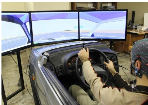
Fig. 1: Snapshot of the car-driving simulator used for the implementation of the proposed protocol
