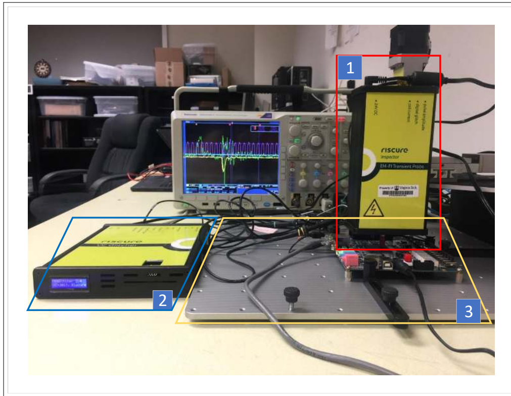
Figure 3.1: 1. EMFI Transient Probe 2. VC Glitcher and 3. XYZ Motorized table
