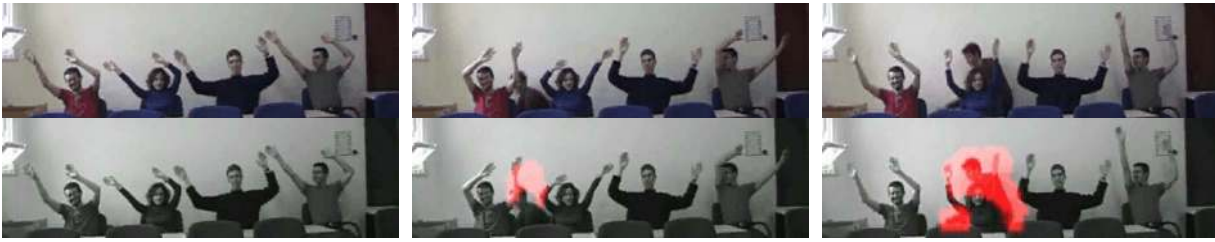
Figure 8. Detecting salient behaviors in a video sequence (no database and no prior information). Saliency is measured relative to all the other behaviors observed at the same time. In this example, all the people wave their arms, and one person behaves differently. For full videos see www.wisdom.weizmann.ac.il/~vision/Irregularities.html
