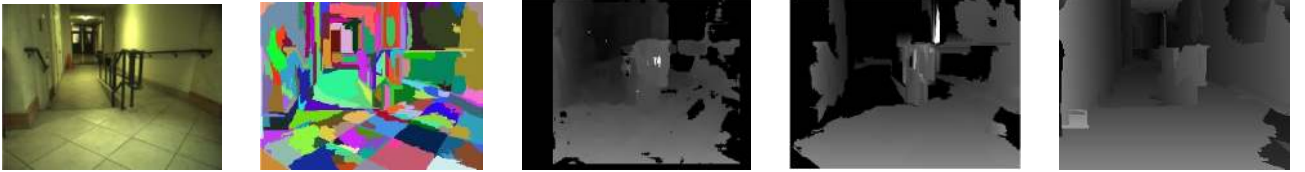
(a) Left image of stereo pair. (b) Color segmented left image. (c) Correlation stereo disparity map of left image. (d) Disparity map after fitting world planes. (e) Disparity map after energy optimization.
