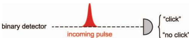
Figure 6. Avalanche photodiodes (APD) are binary detectors. They exhibit single-photon sensitivity, but can only measure if any light is present not how many photons are incident.
