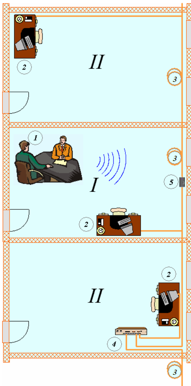
Figure 6. Schematic diagram of protection against leakage information through fiber optic communications, based on detector of attack. I: allocated room; II: secondary rooms. 1: location of confidential negotiations; 2: workplace (workstation); 3: fiber optic communications; 4: regular active optical network equipment; 5: inclusions detector attack.
