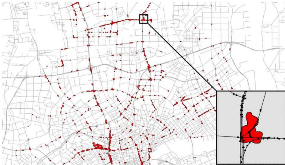
Figure 9. Selection of TIP polygon in the north of Shanghai based on taxi FCD from 8:00 to 9:00 am on 22 February 2007.
