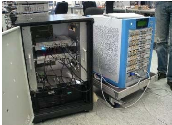
Fig 62. The measurement configuration consisting of a Propsim C8 channel emulator on the right and a RACE platform on the left.
