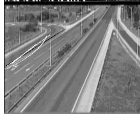
Fig. 15. Performing a similarity search under the d_{\min} distance function with a user-specified query. Retrieved vehicle trajectories are displayed.
