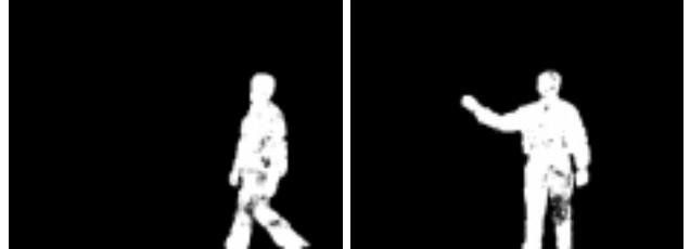
Figure 6. Combined subtraction results after median filtering for frames 125 and 225 of the sequence in Figure 1.
