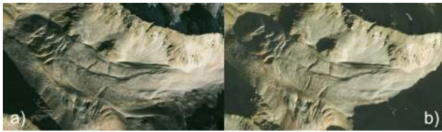
Figure 2. This figure shows a temporally mixed stereogram of Hinteres Langtalkar rock glacier at 80 cm GSD. a) Screen shot of Google Maps, image acquisition date: 18 September 2002, image source: aerial photograph, BEV. b) Screen shot of Microsoft Bing Maps, image acquisition date: 21 September 2006, image source: aerial photograph, Province of Tyrol. Surface deformation can be perceived quite well in the stereogram due to the large horizontal parallaxes introduced by the right-to-left movement of the rock glacier. Also notice the development of tension cracks in the permafrost body.
