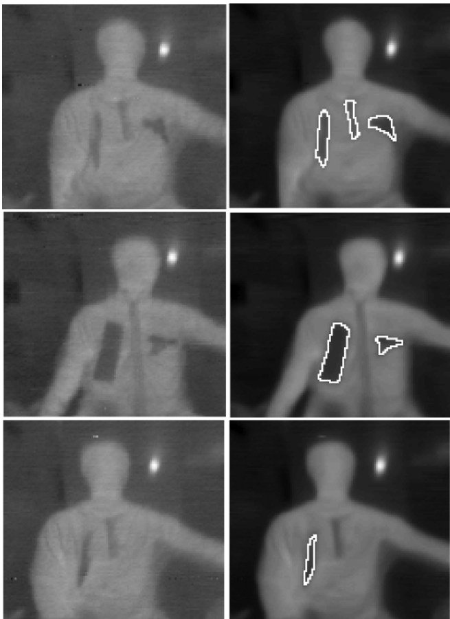
Fig. 11. Left: original images (1, 2, and 3 from top to bottom); right: segmentation of the concealed objects detected by our algorithm.
