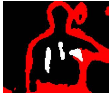
Fig. 7. Set of pixels with intensity in [T_{low}, T_{high}] is partitioned into P_b and P_c . Pixels in P_b (shown in red) are located at the boundary of the human body. Pixels in P_c (shown in white) belong to the concealed objects.
