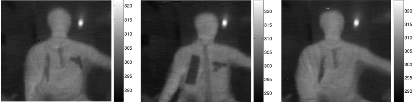
Fig. 1. Image 1 (left), T \in [285.84, 322] . A ceramic knife and a handgun are concealed under the clothing. Image 2 (center), T \in [286.67, 324] . A handgun and a rectangular piece of standard RF anechoic material are concealed under the clothing. Image 3 (right), T \in [285.88, 324] . A ceramic knife is concealed under the clothing. The radiometric temperature T is mapped to grayscale intensity.
