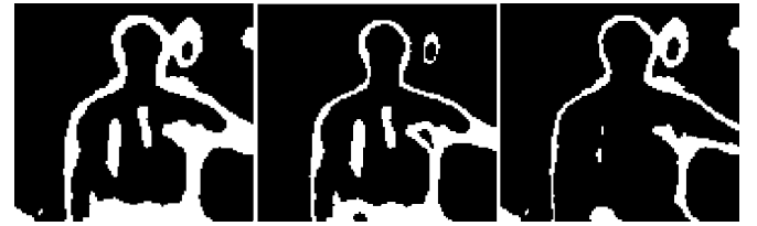
Fig. 3. Pixels i such that I(i) is in given range. Left: range = [T_{low}, T_{high}] . Center: range = [T_{low} + \delta, T_{high}] . Right: range = [T_{low}, T_{high} - \delta] . We have T_{low} = 295.37 K, T_{high} = 303.35 K, and \delta = 3 K.
