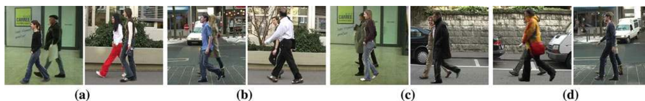
Fig. 3 Examples of synthetically generated training images for different levels of occlusion: 5–10 % (a), 20–30 % (b), 40–50 % (c) and 70–80 % (d)
