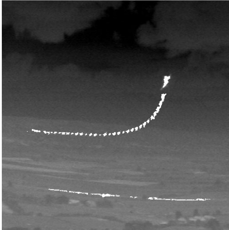
Figure 7: The whole sequence of tracked objects superimposed upon the last image of the sequence to give an idea of the motion and shift in target sizes.
