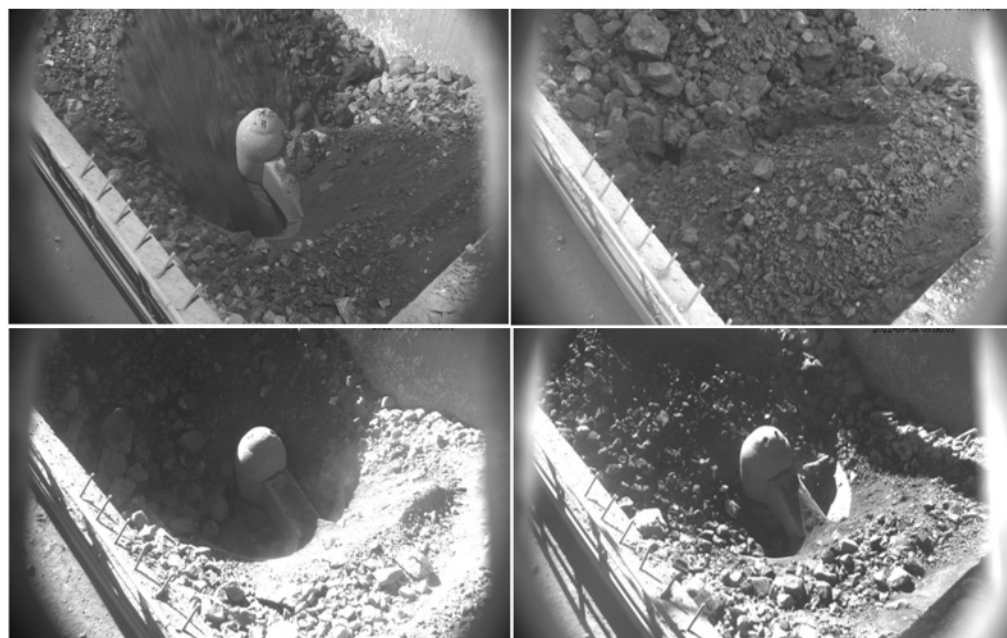
Figure 10. Crushing mouth blockage.
