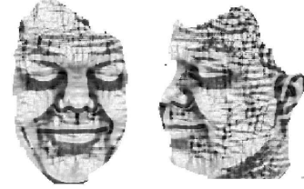
Figure 5. Example shape index images. The dark regions correspond to a shape index of 0 while the lighter regions represent a shape index of 1.
