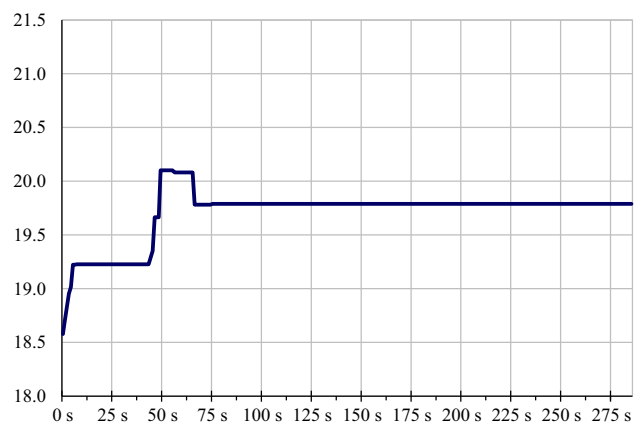
Fig. 13 RAM usage (MB) by the proposed IDS in the virtual machine stress test as a function of time
