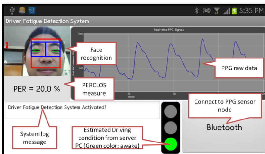
Figure 6. Screenshot of a smartphone that shows the measurement of the PERCLOS, the display of raw PPG data, and the estimation of the driver's level of alertness.
