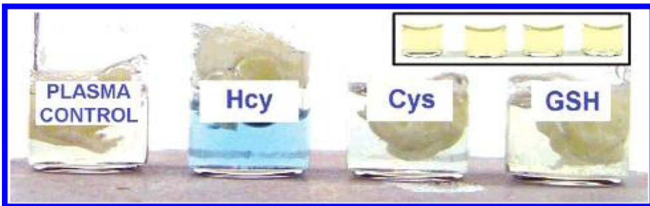
Figure 6. Selective Hcy detection in human plasma without prior deproteinization. Only the Hcy-spiked sample turns blue (added thiol left to right: none, Hcy, Cys, GSH, 4.0 mM final thiol concentration). Inset: samples before heating.
