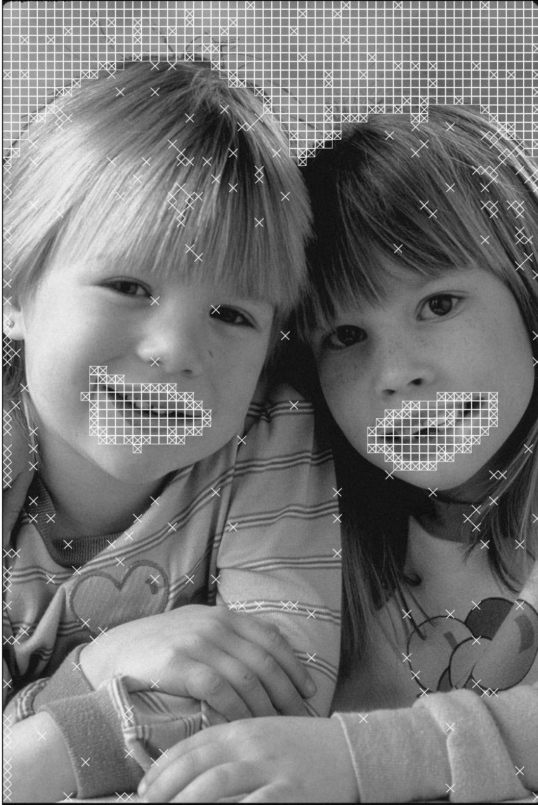
Figure 7: Illustration of Detection Performance ( \sigma=5.0 , T=0.1 , blocksize=16x16, JPEG-60 bitrate=0.90 bpp, 93% correct detection, 4% false positive, 17% misses.) A box indicates an altered block correctly identified, X indicates false positive, and X within a box indicates a miss.
