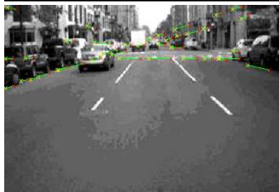
(c) Results with Canny edge detection and its Hough transform
