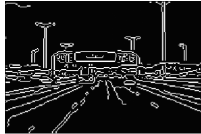
(b) Result with variable thresholding
