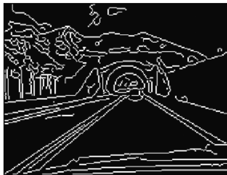
(a) Result with variable thresholding
