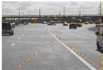
(c) Results with Canny edge detection and its Hough transform
