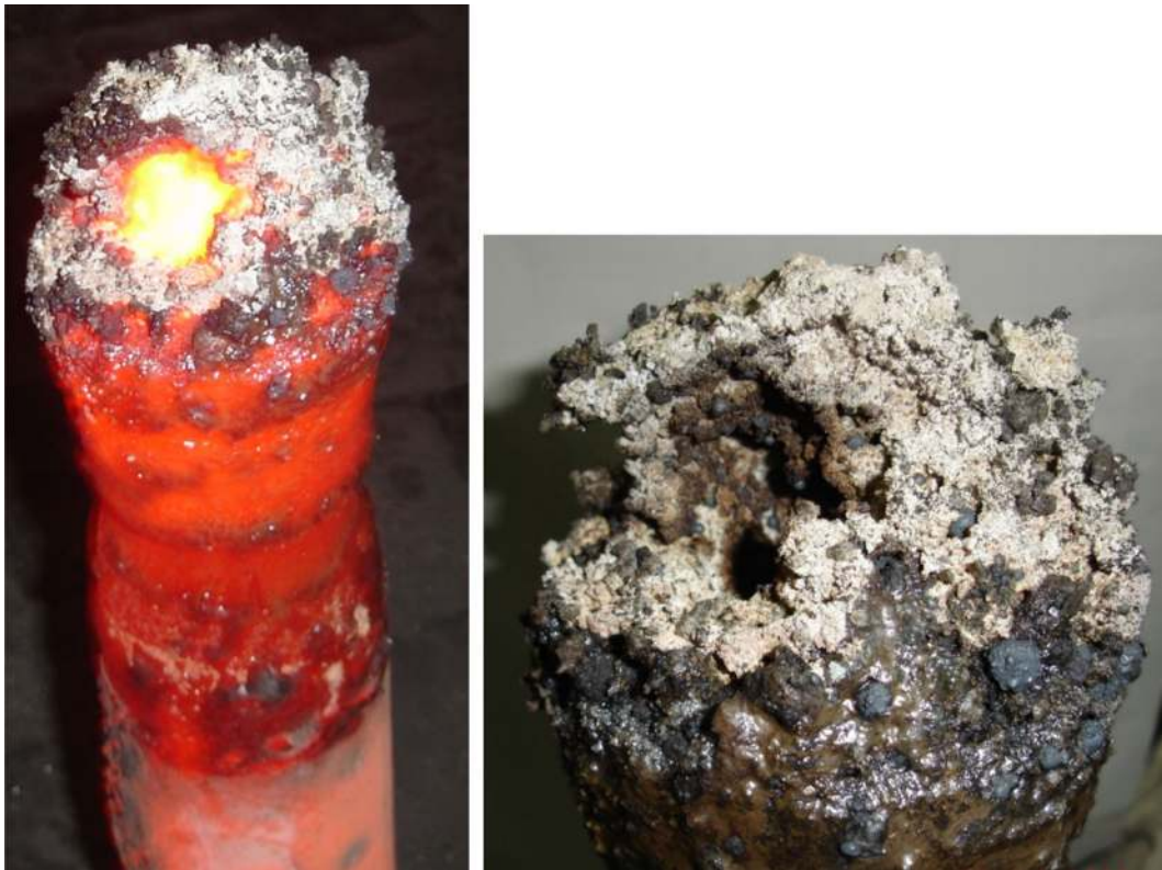
Fig. 7—Clogging materials (mainly Al 2 O 3 -CaO-MgO inclusions) at the submerged entry nozzle.
