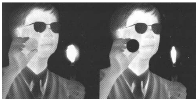
Fig. 42. Simultaneous images from 256 \times 256 MWIR/LWIR QWIP FPAs. Note appearance of the front-held filter and the hot soldering iron in the two bands. Reproduced from [31]
