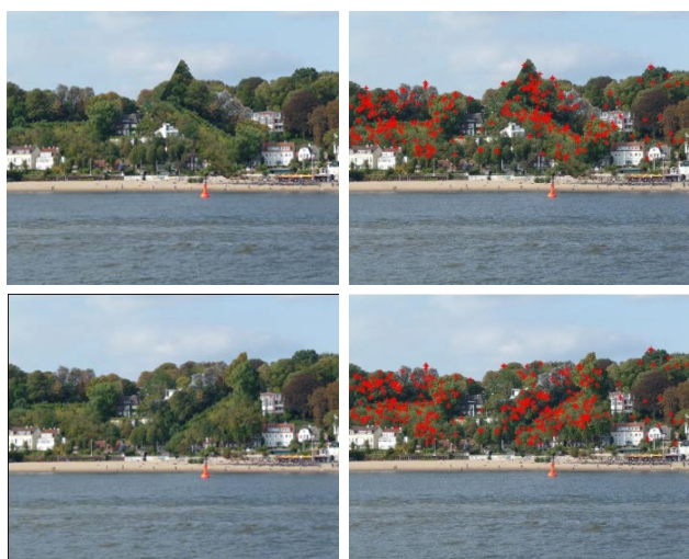
Fig 10. Copied region rotated in angle 30 degree clockwise (upper left) and the detected result (upper right) and the tampered region is rotated 30 degree anticlockwise (bottom left) and the detected result (bottom right).
