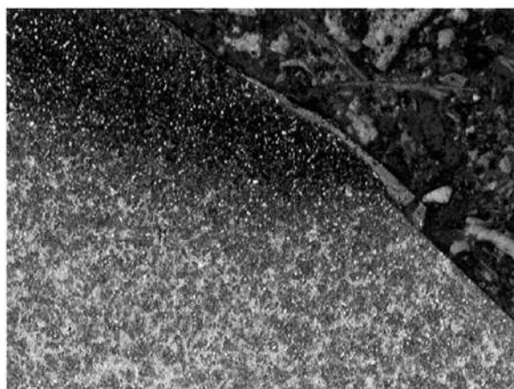
Fig. 15 Sliding test wear scar, 100\times
