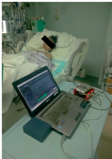
Fig. 6. Measurement environment. The device is connected to the tube of ventilator near the mouth of a patient. The respiratory sounds are measured by the sound sensor and then transformed into a digital signal by the audio card at a sampling rate of 44 100 Hz
