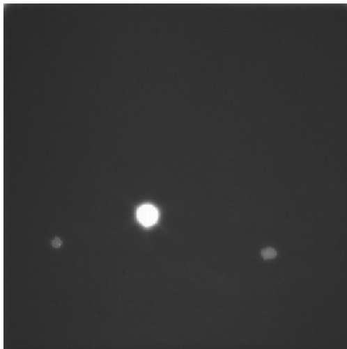
Fig. 8. Natural CMOS anti-blooming behavior demonstration (the two gray spots response is at mid-dynamic range level while the white one is over saturated).
