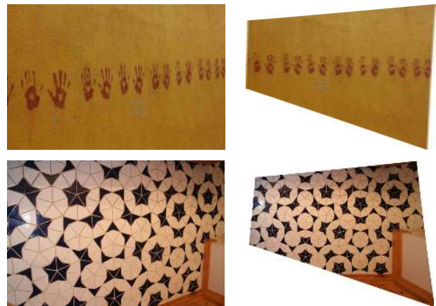
Figure 1. Two different repeated patterns (left column) detected and used to rectify the images (right column) by the proposed algorithm. Top: similarity rectification with scale ambiguity in the vertical axis from a pattern with reflected elements; bottom: similarity rectification from an irregular pattern with rotated elements—note the right angle of the corner in the rectified image.
