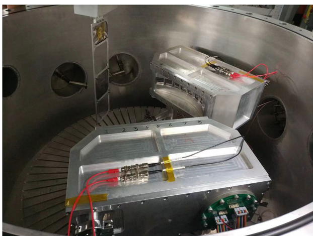
Fig. 14 Photo of LPDA at Back-n. Sixteen telescopes are divided into two identical parts; the target holder is at the center of the vacuum chamber
