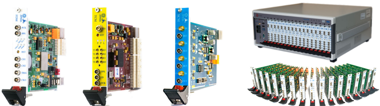
Fig. 32 Photography of electronics modules (from left to right: FDM, TCM, SCM and readout crate)
