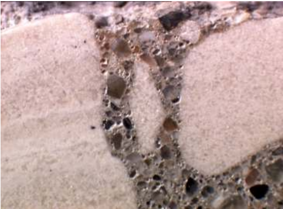
Figure 10. Iowa 175 Core 2 surface microstructure. Slight discoloration in the upper mortar indicates approximate depth of carbonation. Micrograph field width: 14 mm
