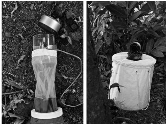
Fig. 1. (A) View from above of the miniature CDC-light trap version of the sound trap as used in the field; (B) picture of a BG trap with portable speaker, placed by a swarm site.
