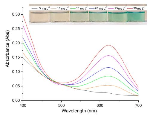
**Figure 5.** UV–Vis spectra of the colored product obtained from the reaction of  $Cr(CO)_6$  with 2AP at different concentrations.
