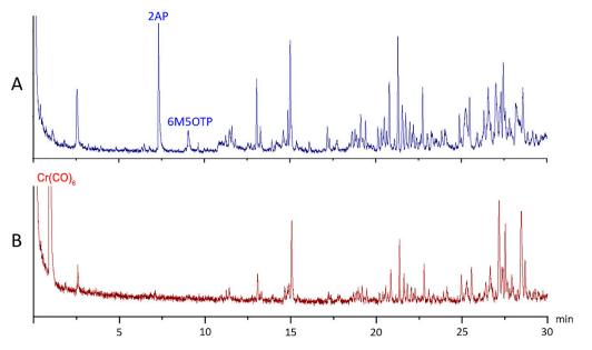
**Figure 3.** GC–MS chromatogram of a fragrant rice extract before (A) and after (B) the addition of  $Cr(CO)_6$ .
