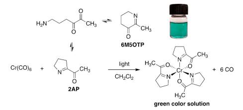
**Figure 1.** Possible mechanism for the light-assisted complexation of  $Cr(CO)_6$  and 2AP.
