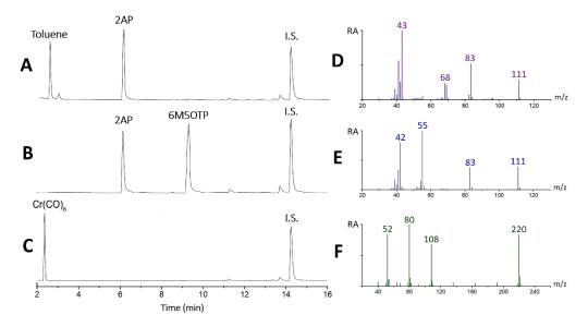
**Figure 2.** GC–MS chromatogram of synthetic 2AP in toluene (**A**), DCM (**B**) and after the addition of  $Cr(CO)_6$  (**C**). Mass spectrum of 2AP (**D**), 6M5OTP (**E**) and  $Cr(CO)_6$  (**F**).
