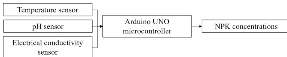
Figure 2 System instrumentation architecture in the sensor-based acquisition of physical limnological data.
