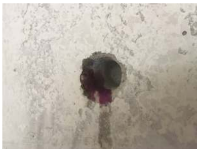
Fig. 4. Color change of phenolphthalein solution due to carbonation of concrete to a depth of 20 mm, according to autopsy No. 4.
