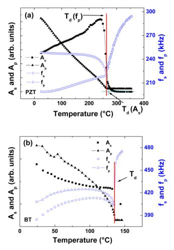
FIG. 10. (Color online) Peak area  $A_s$  and  $A_p$  and frequency of serial and parallel resonance  $f_s$  and  $f_p$  for (a) PZT, and (b) BT (at the transition only data for parallel resonance was taken). The vertical line denotes  $T_d$  determined by the minimum of  $f_p$ .
