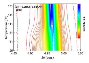
FIG. 12. (Color online) In situ temperature dependent x-ray diffraction of (200) reflection in (BNT–0.2BKT)–0.02KNN. The tetragonal splitting of the peak visible by the broader intensity on the low  $2\theta$  part of the peak vanishes around  $102 \,^{\circ}$ C leading to a single peak.
