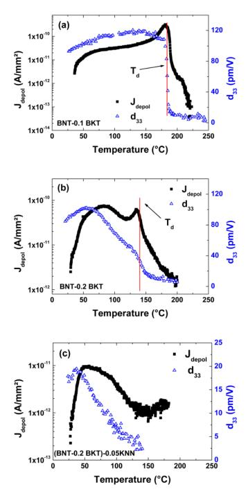
FIG. 6. (Color online) Temperature dependence of piezoelectric coefficient  $d_{33}$  and depolarization current  $J_{depol}$  for (a) BNT–0.1 BKT, (b) BNT–0.2 BKT, and (c) (BNT–0.2BKT)–0.05KNN. The vertical line denotes  $T_d$ , determined by  $d_{33}$ .
