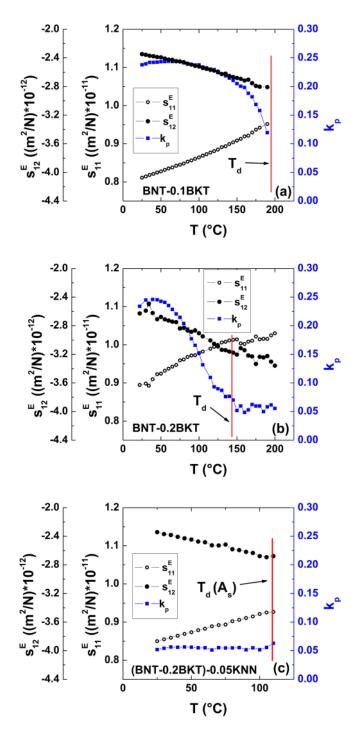
FIG. 14. (Color online) Elastic compliance  $s_{11}^E$  and  $s_{12}^E$  and planar electromechanical coupling factor  $k_p$  for (a) BNT–0.1BKT, (b) BNT–0.2 BKT, and (c) (BNT–0.2BKT)–0.05KNN. The vertical line marks  $T_d$  determined by the minimum of  $f_p$  if not specified otherwise.
