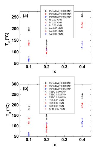
FIG. 15. (Color online) Comparison of  $T_d$  of (BNT–*x*BKT)–*y*KNN ceramics derived from inflection point of permittivity to  $T_d$  determined from (a) minimum in parallel resonance frequency  $f_p(T)$  and the temperature where the resonance peak area  $A_s$  vanishes, and (b) peak in TSDC, steepest decrease in  $d_{33}(T)$  and change in (200) peak determined by high-energy in situ XRD.
