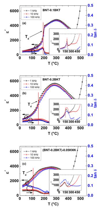
FIG. 8. (Color online) Dielectric permittivity  $\varepsilon'$ , dielectric loss tan $\delta$ , and imaginary part of dielectric permittivity  $\varepsilon''$  for (a) BNT–0.1 BKT, (b) BNT–0.2BKT, and (c) (BNT–0.2BKT)–0.05KNN. The vertical line marks  $T_d$  determined by the inflection point of permittivity.
