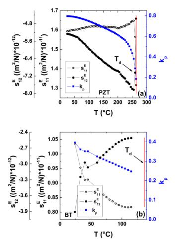
FIG. 13. (Color online) Elastic compliance  $s_{11}^E$  and  $s_{12}^E$  and planar electromechanical coupling factor  $k_p$  for (a) PZT, and (b) BT. The vertical line denotes  $T_d$  determined by the minimum of  $f_p$ .
