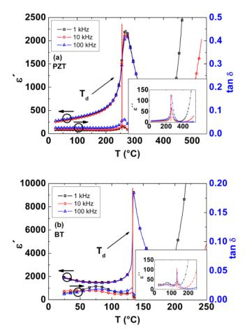
FIG. 7. (Color online) Relative dielectric permittivity  $\varepsilon_r$  and dielectric loss tan $\delta$  for (a) PZT, and (b) BT. The vertical line denotes  $T_d$  determined by the inflection point of permittivity.
