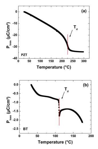
FIG. 3. (Color online) Polarization loss calculated from TSDC measurements for (a) PZT, and (b) BT.
