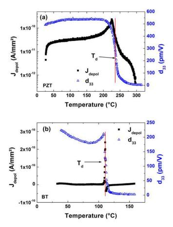
FIG. 5. (Color online) Temperature dependence of piezoelectric coefficient  $d_{33}$  and depolarization current  $J_{depol}$  for (a) PZT, and (b) BT. The vertical line denotes  $T_d$ , determined by  $d_{33}$ .
