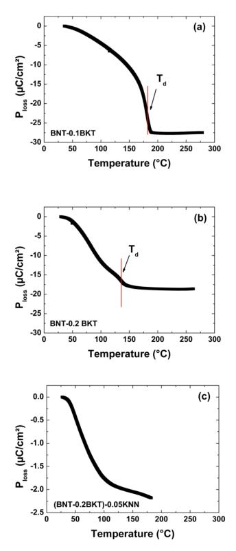
FIG. 4. (Color online) Polarization loss calculated from TSDC measurements for (a) BNT–0.1BKT, (b) BNT–0.2BKT, and (c) (BNT–0.2BKT –0.05KNN.
