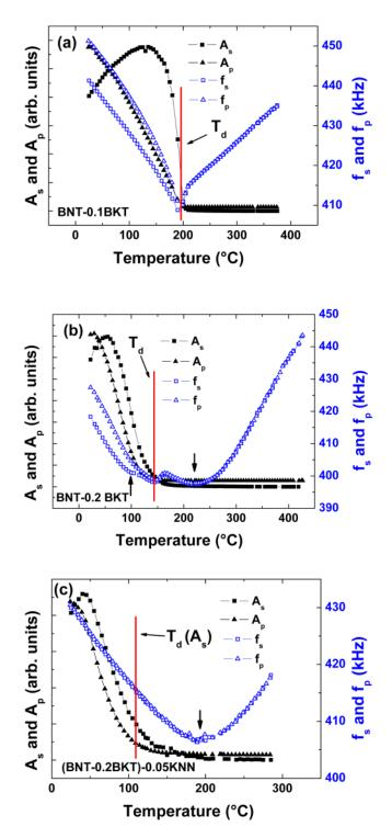
FIG. 11. (Color online) Peak area  $A_s$  and  $A_p$  and frequency of serial and parallel resonance  $f_s$  and  $f_p$  for (a) BNT–0.1BKT, (b) BNT–0.2 BKT, and (c) (BNT–0.2BKT)–0.05KNN. The vertical line denotes  $T_d$  determined by the minimum of  $f_p$  if not specified otherwise.
