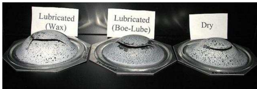
Figure 12: Effect of friction on formability of full width specimens.
