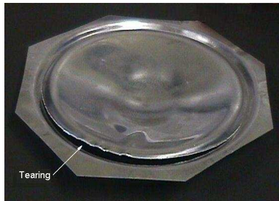
Figure 2: Tearing of Al2524-T3 specimen at lock-bead during the test.
