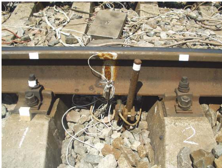
Figure 5. Installing transducers on a rail
