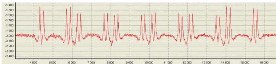
Figure 6. Example of rail stress record (stress on the base edge due to Skoda train passing at a speed of 176 km/h)
