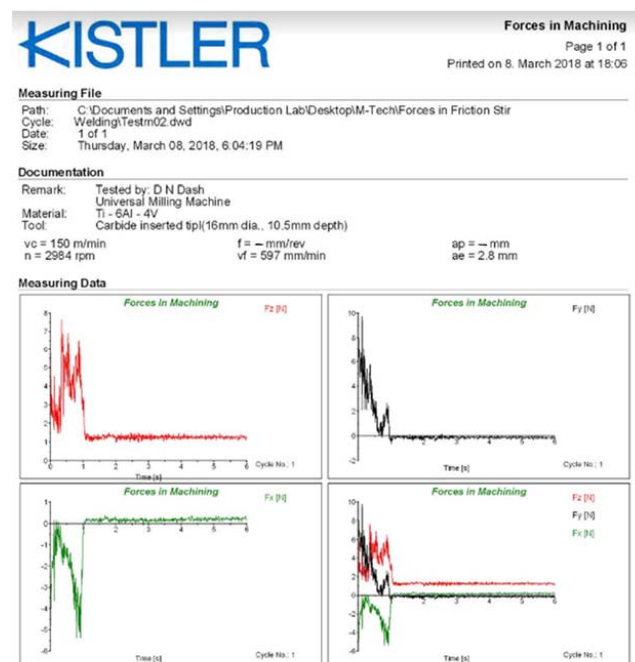
Figure 5. Reading obtained using tool dynamometer for various components of forces.
