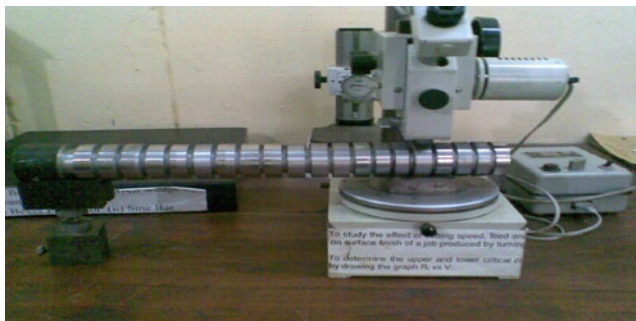
Fig. 2 Surface roughness-measuring microscope with workpiece EN-31 steel
