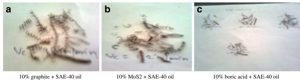
Fig. 3 Chips produced with different lubricant during experiments. a 10% graphite + SAE-40 oil, b 10% MoS 2 + SAE-40 oil, c 10% boric acid + SAE-40 oil
