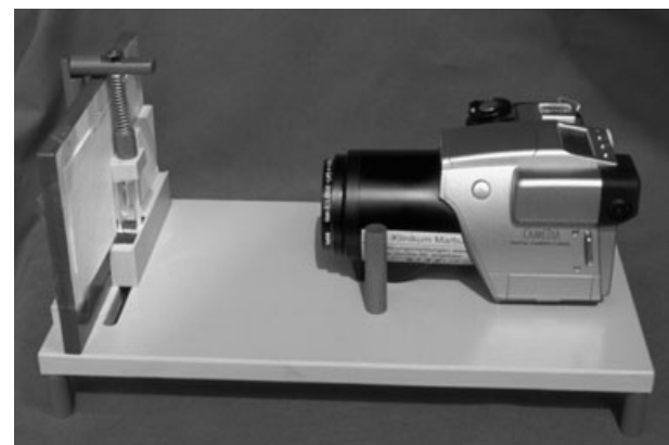
Figure 1 Purpose-designed stand for standardised photograph.
