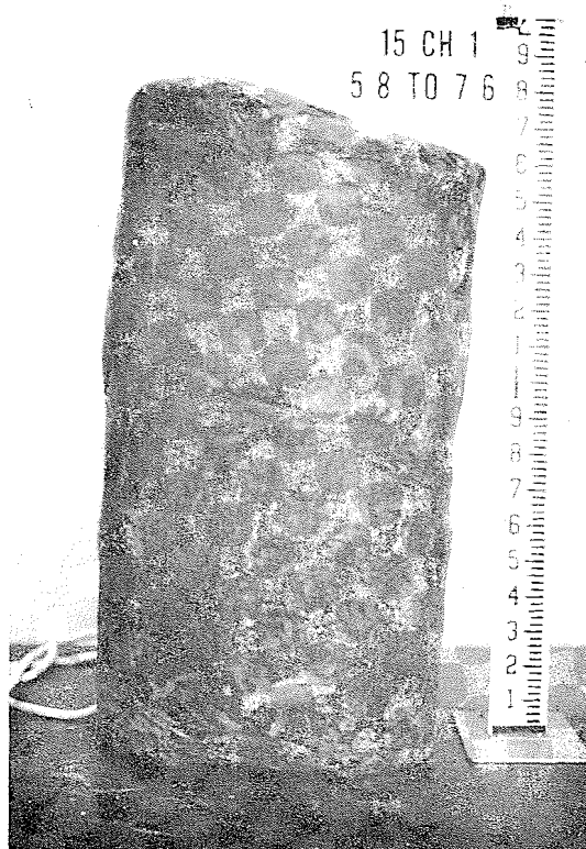
FIG. 2. Large diameter sample (15-CH-1, 5'8"-7'6") as received at the laboratory.
