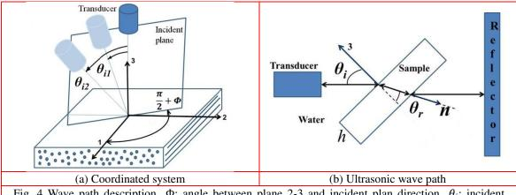
Fig. 4 Wave path description.  $\Phi$ : angle between plane 2-3 and incident plan direction.  $\theta_i$ : incident angle.  $\theta_r$ : refraction angle
