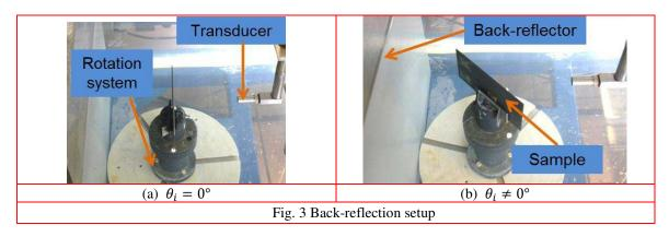
The measurements are performed for different angles  $\Phi$  between plane 2-3 and incident plane (see Fig. 4). For a given  $\Phi$ , the sample is then rotated in the incident plane for different incident angles  $\theta_i$  between the transducer and axis 3 of the sample. The wave passes through the sample in the direction of n with angle  $\theta_r$ , so  $\theta_r$  is function of  $\Phi$  and  $\theta_i$ . For each set of angles ( $\Phi$  and  $\theta_i$ ), the time of flight is measured.
