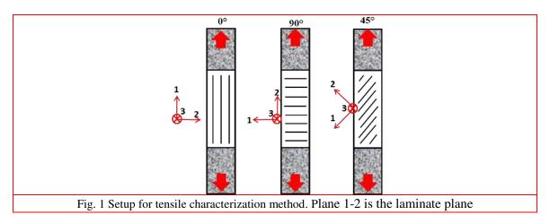
Mechanical tests are carried out at ambient temperature in a room thermoregulated at 25 °C. Uniaxial tensile tests are performed by an electromechanical testing machine INSTRON 5500. According to the standard, the displacement rate is 2 mm/min for 0° samples, 1,5 mm/min for 45° samples and 1 mm/min for 90° samples. To check the reproducibility of the response, three specimens are considered for each loading direction.
